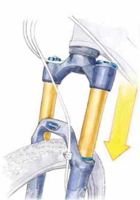
1. Add recommended air for rider weight (see chart on facing page). With bike on level ground, bounce up and down a bit to overcome stock stiction. Settle into your riding position.
