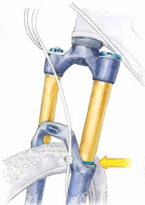
2. Slide o-ring until it rests on wiper, then dismount without disturbing o-ring's position.
