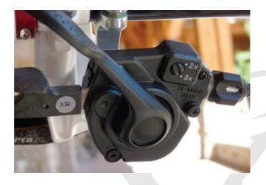
For SRAM shifting, the shifter is dedicated to double or triple chainrings. Either will work. We use a double shifter with a triple derailleur since the first shift (from inner to whatever next chainring) uses the same cable pull. A triple front shifter will also work. The use of a triple front derailleur is crucial.
