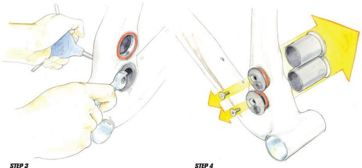
Remove the countersunk bolt from each eccentric core cap. You might need to use a 12mm open end wrench to prevent the eccentric from rotating. Do not use a crescent wrench, cave man!
