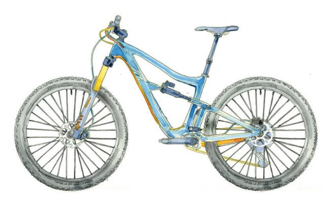
**IMPORTANT:** Before riding, check the saddle to tire clearance with the dropper post fully dropped and the air out of the shock with frame compressed to bottom out.
