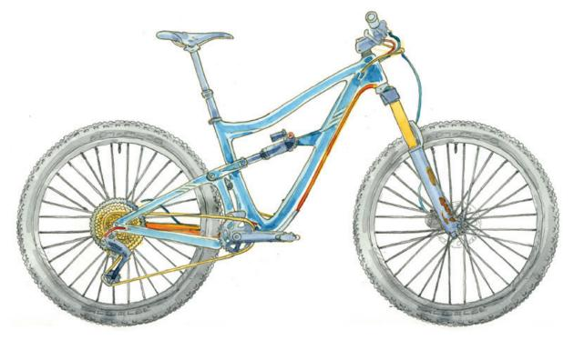
For cable routing, the Ripmo features carbon fiber tubes molded inside the frame. Just push the housing through and it pops out the other end. Simple! And quiet too.
