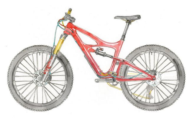
The most common set-up these days is a 1X drivetrain with an internally mounted dropper. We spec the Fox Transfer. We generally recommend you run your brake on the exterior, along the left side of the down tube.
