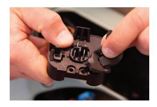
**C.** Use a **T20** Torx key to remove the lower battery cradle from the lower battery mount.
