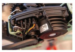
**B.** Rotate the chain guide up and pull the chain off the chainring. Remove the motor using a **6mm** Allen key.
