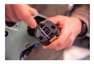
**D.** Install the clamp ring cradle on the battery cradle.
