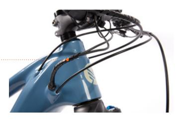
We do not recommend putting the shifter dropper housing in the loom with the e-wires. If they're all together, the dropper housing tends to pull the wire grommet out of the frame.
